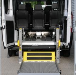
The wheelchair enters the vehicle via the lift; the AMF-Bruns PROTEKTOR system secures person and wheelchair.
