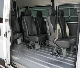
The SMARTFLOOR system floor allows flexible transport of people with and without wheelchairs
