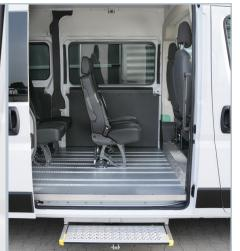
Electric step and handle on the side entry provide easy access to the passenger compartment.
